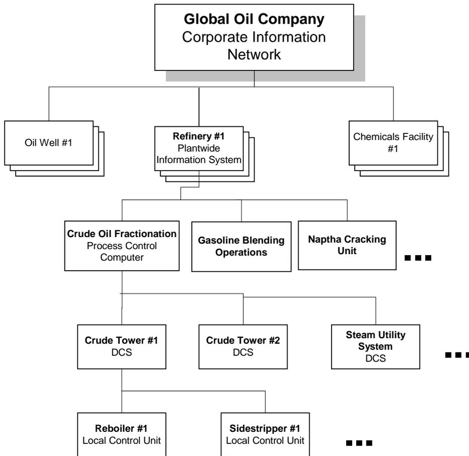
**Figure 1.5** Geographical decomposition of the hierarchical control structure as applied to an oil company.
