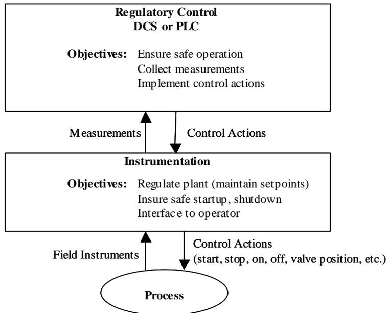
**Figure 1.2** Lower levels of the control hierarchy.
