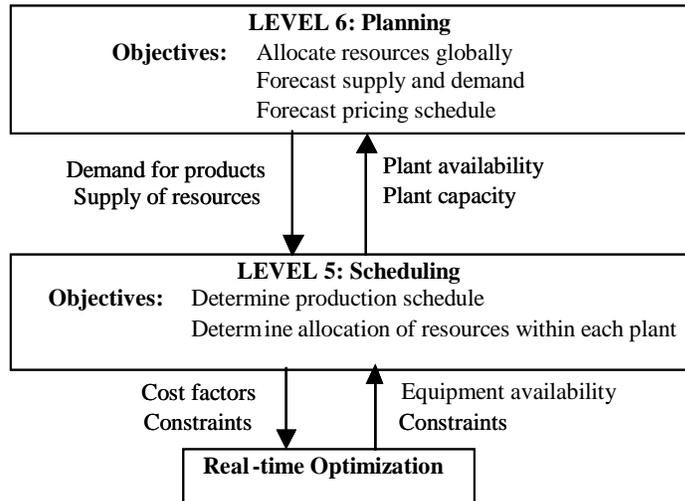
**Figure 1.4** Top layers of the control hierarchy.
