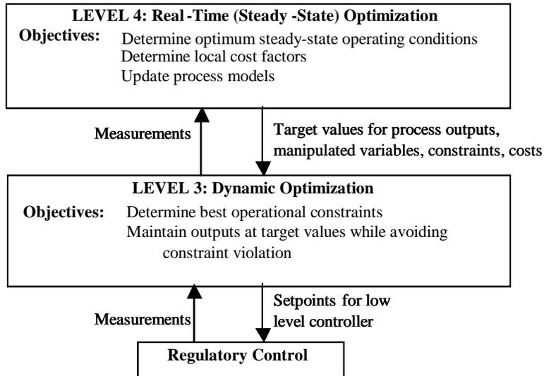
**Figure 1.3** The middle layers of the control hierarchy.
