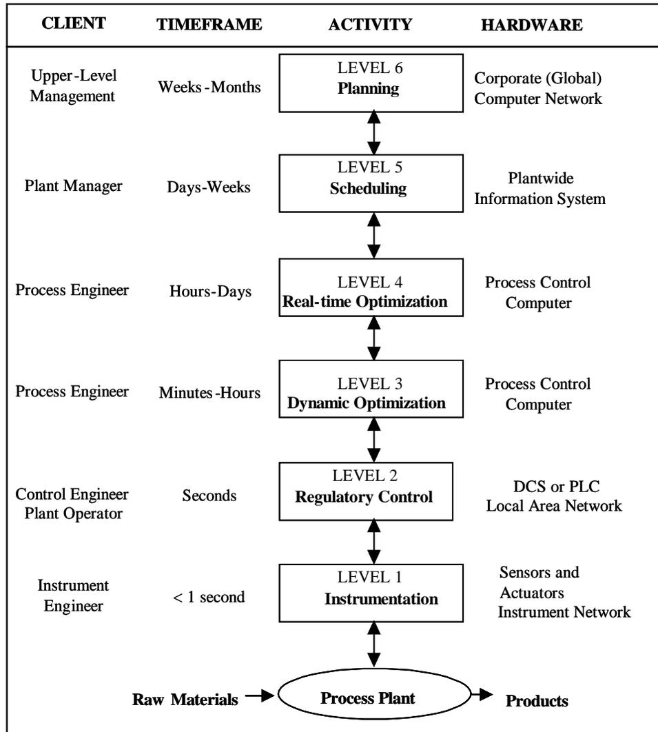
**Figure 1.1** The six-layer hierarchical decomposition of control functions.
